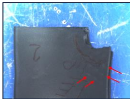
Hpt Blade with Obstruction of Cooling Hole
